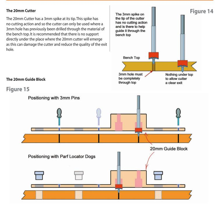
The 20mm holes are created using the 20mm Guide Block, the special 20mm cutter and either the 3mm Guide Pins or the Parf Locator Dogs.
