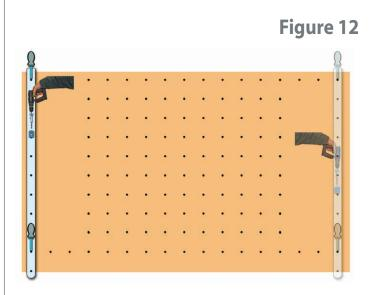
Once the top row has been extended to the left and right perform a similar operation for the lower area shown at B (1st) and B (2nd). Then complete the new columns with a single Parf Stick, held by two 3mm Pins in a similar fashion to that shown in Figure 10 which completes the blue and green area of holes.
